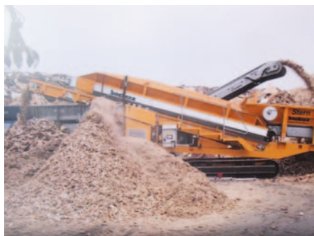
Screening of old wood after upstream coarse crusher
