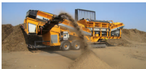
Finest starscreen technology: Wood chips screening with fine fraction 0 - 5 mm
