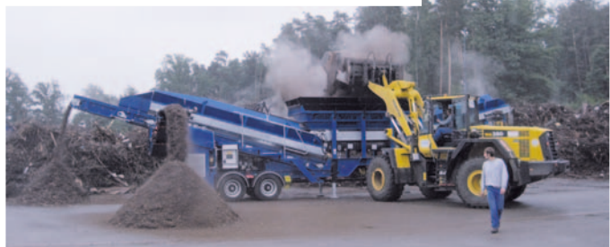
Screening of compost in 3 fractions
