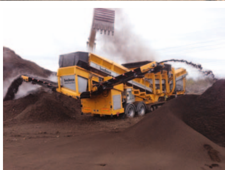
Screening of mulch in 3 fractions
